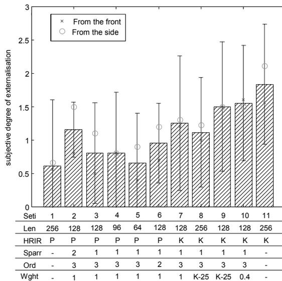
Fig 7: Subjective degree of externalisation for each setting. Depicted values are given for directions from the front, the side and a mean of both of them, where *Seti* is the setting, *Len* is the filter length, *HRIR* is the kind of HRIR-set used (*P*: proprietary, *K*: KEMAR), *Sparr* is the number of speakers near the median axis, *Ord* is the number of ambisonic order and *Wght* is the weighting of ambisonic orders.
